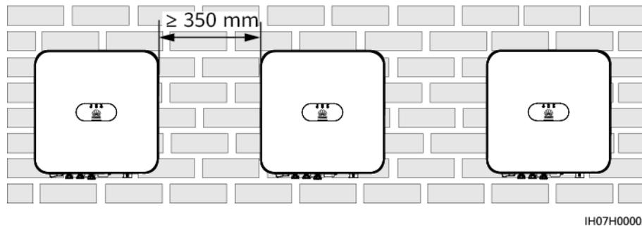
**Figure 4-4** Triangle installation mode (recommended)
