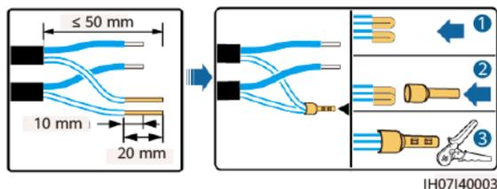
Figure 5-24 Crimping three signal cables
