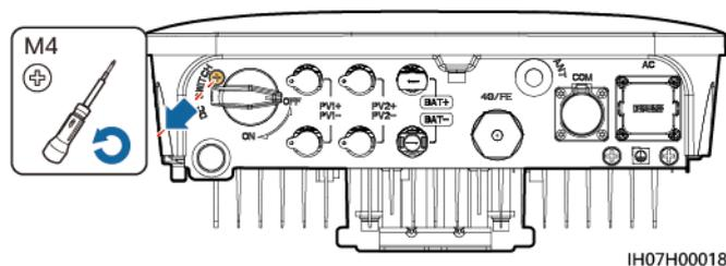
**Step 4** Turn on the DC switch between the PV string and the SUN2000 if there is any.
