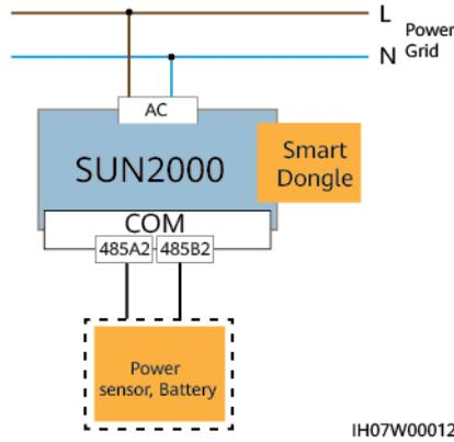
**Figure 5-20** Connecting cables to the smart power sensor (single SUN2000)
