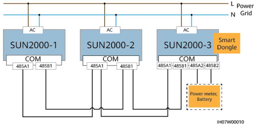
Figure 5-22 Connecting cables to the smart power sensor (in-phase grid connection)
