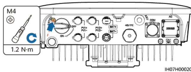
**Step 5** Turn off the DC switch between the SUN2000 and PV strings.
