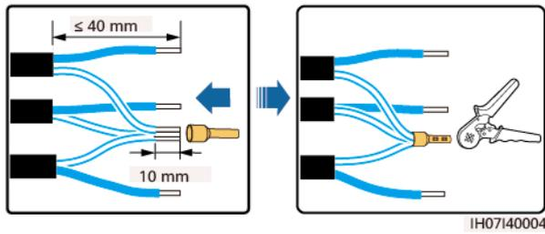
Figure 5-25 Assembling a signal connector (single SUN2000)
